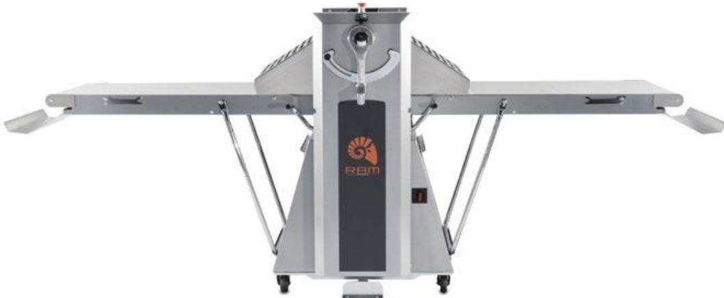
The dough sheeter for excellence. It is provided with a practical and ergonomic direction arm and with a pedals to invert the belts' direction. Its strong structure and large cylinders guarantee an excellent lamination as well as reliability and great durability over time. Q600 also offers the possibility to easily close and remove the table already complete with lower plates. The scrapers, as all the other parts that require a periodic cleaning, are easily accessible by the operator.
